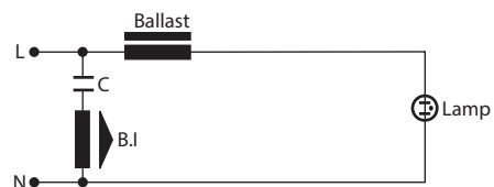
HID lamp circuit with power factor correction capacitor and blocking inductor.
